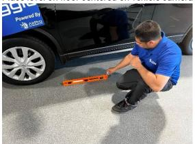
Place inclinometer on level and hold zero button until zeroed.
