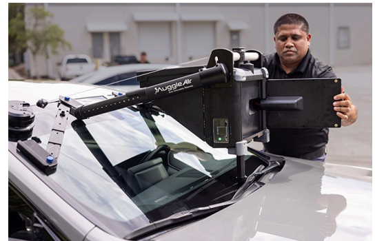
AIRPRO'S AUGGIE AIR DIGITAL TARGETING DEVICE, MOUNTED ON THE WINDSHIELD AHEAD OF A CALIBRATION
