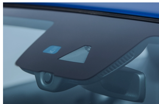
THE FORWARD-FACING CAMERA BEHIND THE WINDSHIELD: THE SYSTEM A STATIC EYESIGHT CALIBRATION IS AIMED AT
